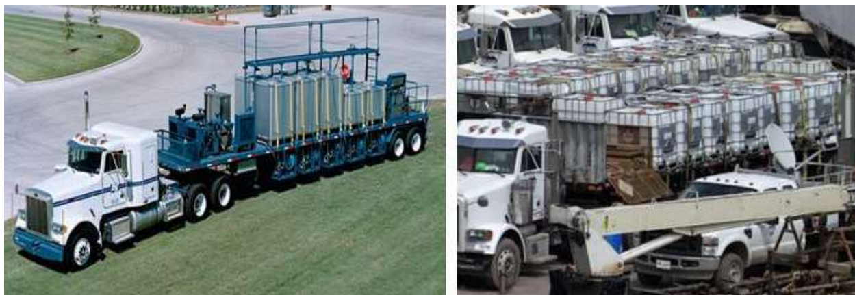
Figure 5-7. Metal and high-density polyethylene (HDPE) additive units.
