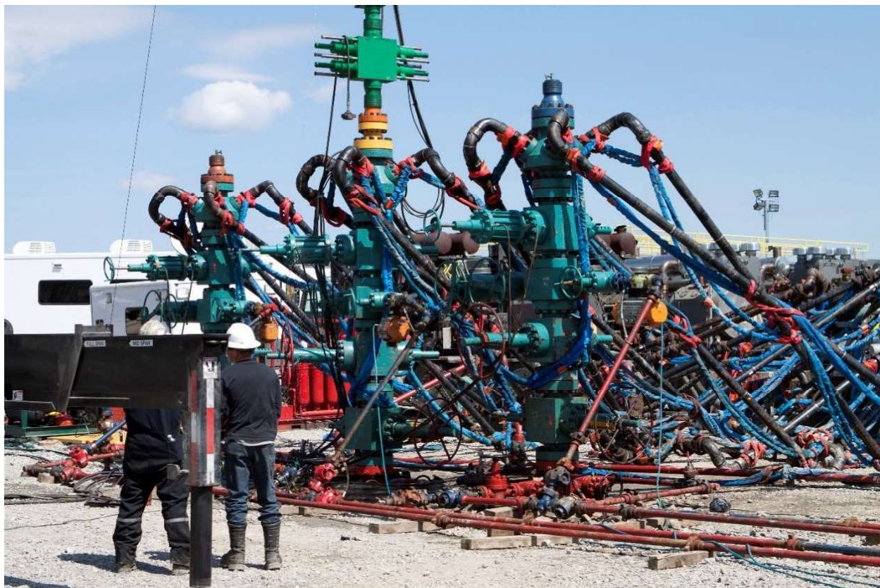
Figure 5-9. Multiple fracture heads.
